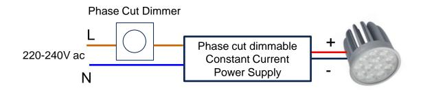
Remark: - 1pc OTe PC driver for 1pc PL-CN50 @350mA - Dimming by reduce output current
